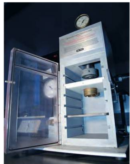
A gene gun or biolistic particle delivery system is a device for injecting cells with genetic information.
