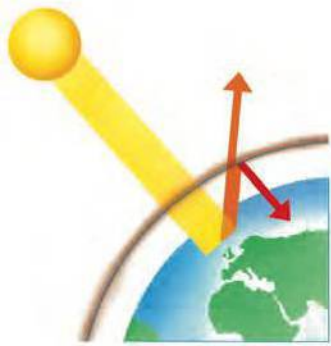
Figure 4.21 A summary of the greenhouse effect: short-wave radiation (shown in yellow) hits the surface and some is converted into long-wave radiation (shown in orange). Some of this infrared heat escapes into space but some (shown in red) is radiated back by greenhouse gases.
